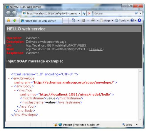
The WSDL URL (in our example <u>http://localhost:1081/nvdef/hello/NVS?WSDL</u>) is available by clicking the "Display it" link from this screen. This URL will be useful for your web service client to automatically construct the messages or code for the web service (e.g. Java AXIS).
